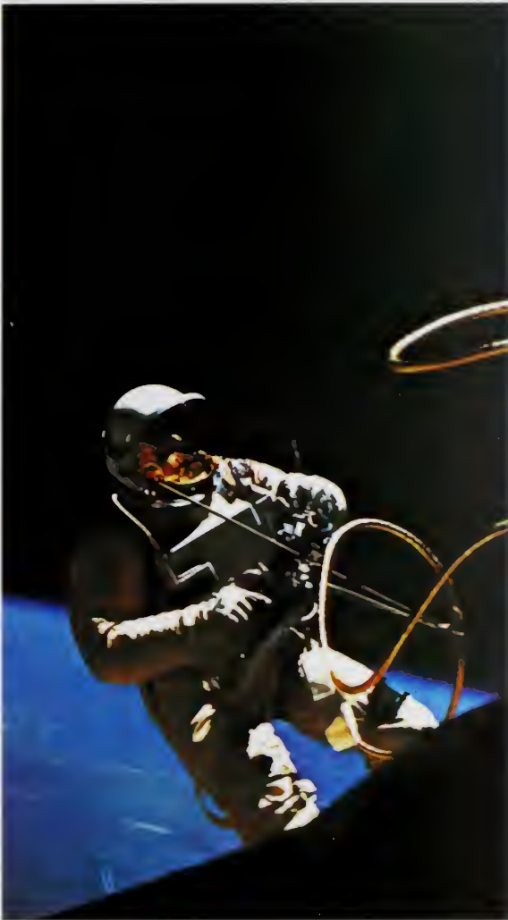
U.S. Gemini 4 astronaut Edward White during his historic 20 minute space walk on June 3, 1965. White was secured to the Gemini spacecraft by an umbilical and tether line and used a maneuvering gun to facilitate movement in space.
